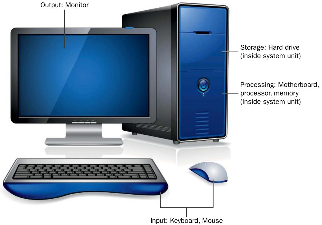
**Figure 1.11** Components of a typical desktop computer system.
